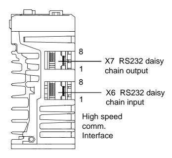
Figure 3-18. Position of Connectors X6 and X7
